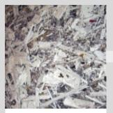
GRP is chopped to granulate by a shreeder.
